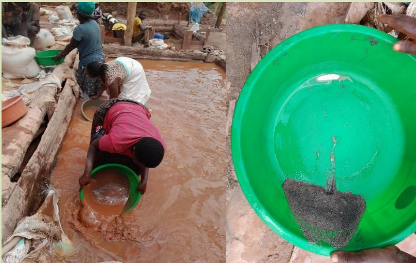
Women washing ore with bare hands and applying mercury without any protective gear in Kasanda District
