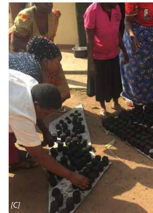
[A] Sorting the ash to remove impurities, [B] Inserting the ash mixed with soil and cassava porridge into the briquettes maker machine, [C] Laying out the made charcoal briquettes in the sun to dry.
