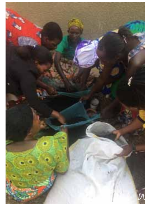
[A] Sorting the ash to remove impurities, [B] Inserting the ash mixed with soil and cassava porridge into the briquettes maker machine, [C] Laying out the made charcoal briquettes in the sun to dry.
