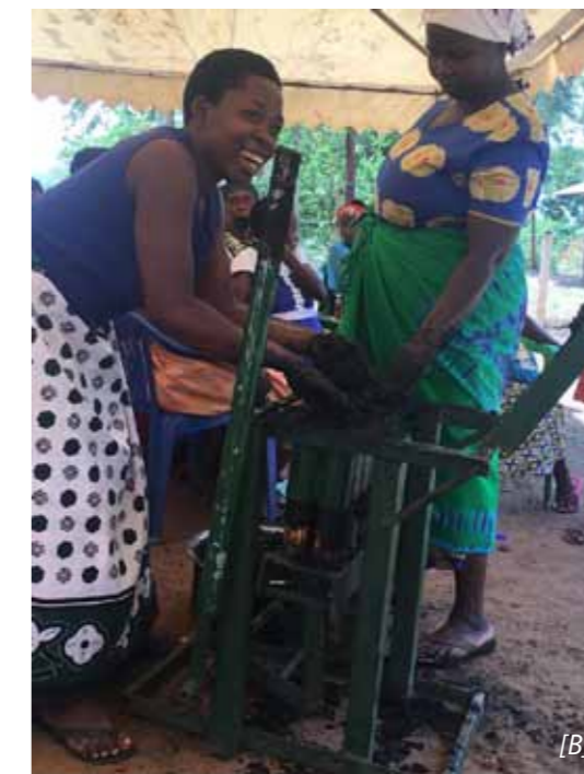
[A] Sorting the ash to remove impurities, [B] Inserting the ash mixed with soil and cassava porridge into the briquettes maker machine, [C] Laying out the made charcoal briquettes in the sun to dry.
